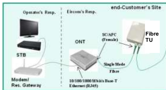
Figure 13: Fibre Demarcation Point for FTTH VUA
