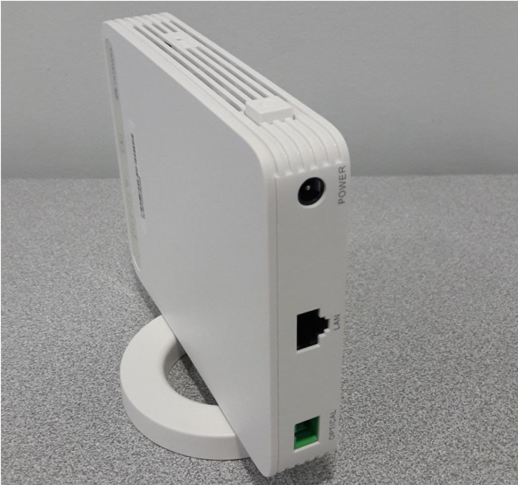
To reset the ONT, the customer needs to insert a pen, pin, paper clip, needle or a similarly shaped object into the reset pinhole located on the top of the ONT for approximately 10 seconds. When the lights on the base of the ONT flash off – the reset has been successful Remember to check Sync and Radius after doing this.
